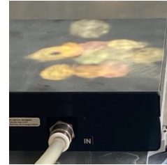
Calorimeter Illuminated with Light Screen Hole Pattern
